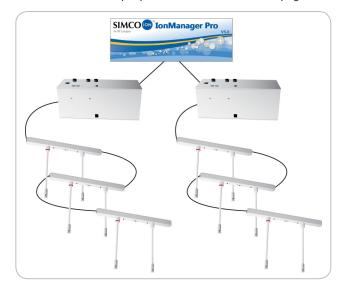
Emitters are connected to the Model 5582 Controllers, which communicate with lonManager Pro to send email notifications to a facility monitoring system or agent.
