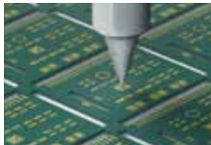
Ag paste dispensing for die bonding
